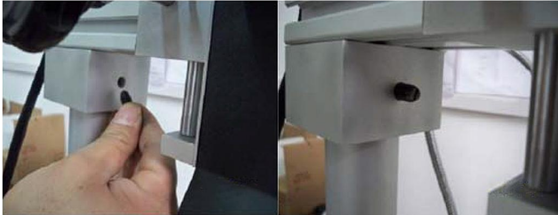
Top head cable connector, RS232, power connector
