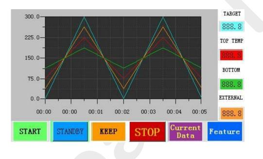
And then will appear top target temperature, top actual temperate, bottom actual temperature, actual thermostatic temperature of the third THERMATIC (preheating temperature at bottom), outer actual temperature from up to down at the right side of the touch screen.
